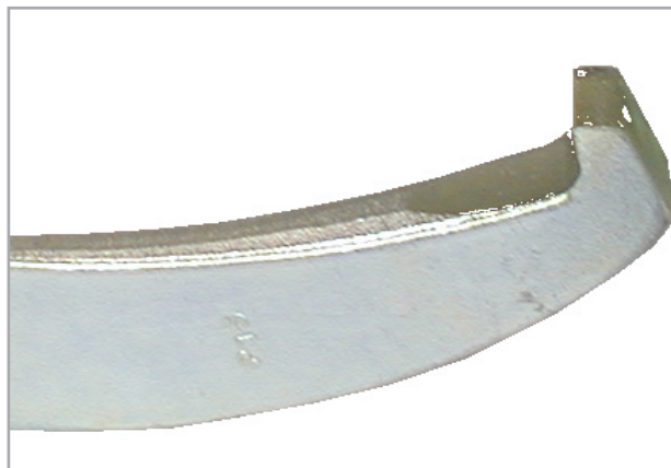
Below: A standard jaw is compared to a specially machined transmission jaw. The transmission jaw tip is .070 inches.
